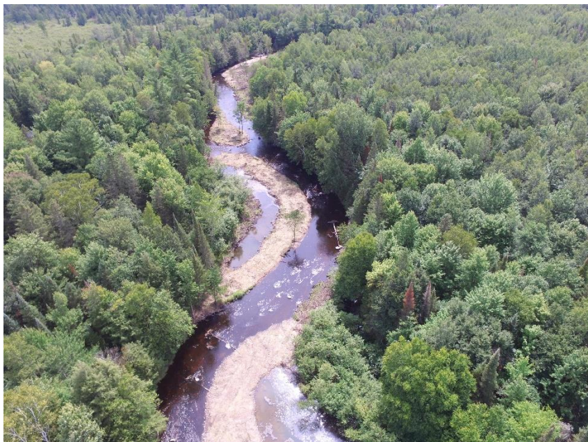
Aerial view of the Prairie River habitat project showing point bar construction, boulder clusters and woody habitat. / Photo credit: Dave Curran
